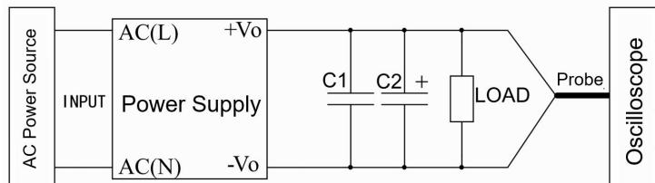
1. The Ripple & Noise test needs the cables in parallel, an oscilloscope that should be set at the Sample Mode, bandwidth 20MHz. 100M bandwidth probe with cap and ground removed. One polypropylene capacitor C1(0.1uF) and one high frequency low impedance electrolytic capacitor C2(10uF) are connected in parallel with the probe.
